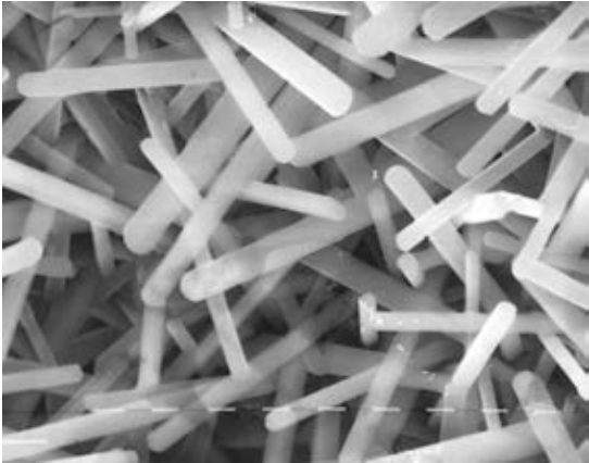
Figure 1.5.10 Fluorcanasite crystals with a large aspect ratio
