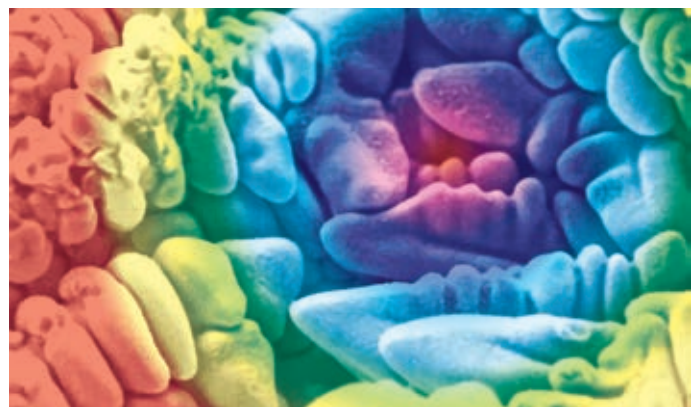
Figure 1.4.14 Scanning electron microscope (SEM) micrograph of the coarse dendritic structure for a CO–Cr alloy
