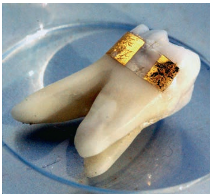
Figure 2.8.9 Graphene sensor deposited on a human tooth. The authors are indebted to Professor Mike McAlpine and his team at Princeton University for this image
